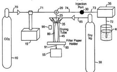
Figure 2: Electronic system for supercritical fluid extraction
