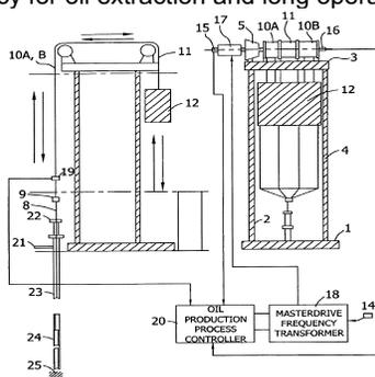
Figure 1: Electronic system of a fully automated machine for oil extraction
