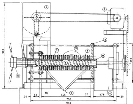
Figure 3: Semi-sectional view of the screw press (oil expeller)
