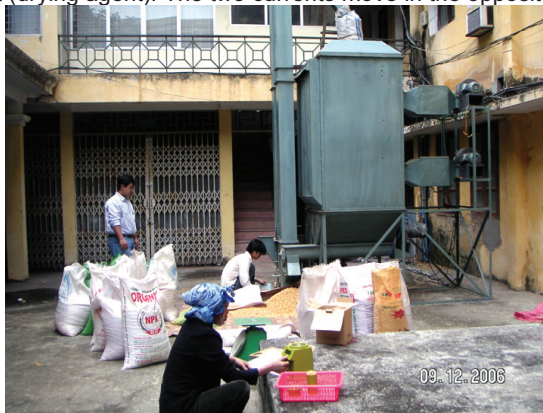
Fig.5. Tower-type corn grain dryer designed by author
