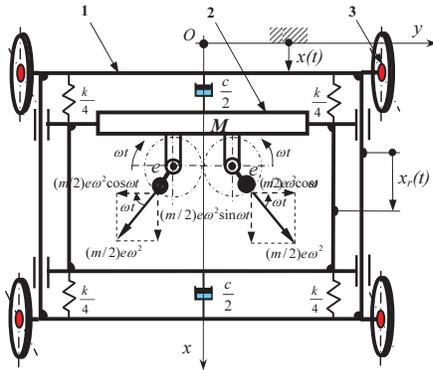
Fig. 13 Dynamic model of the inertial drive
