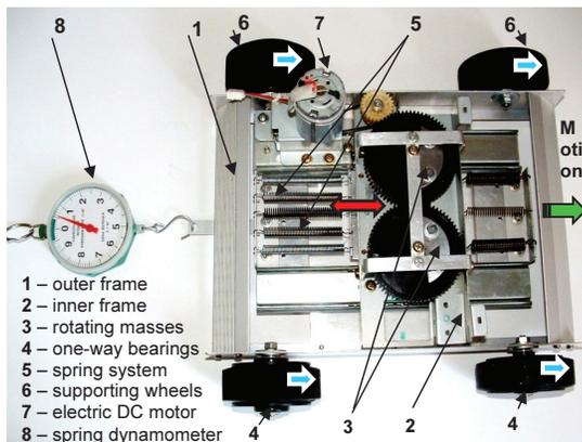
Fig. 12 Top view of the II<sup>nd</sup> inertial drive
