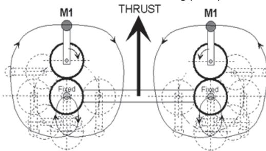
Fig. 3 The mass & thrust diagram of Thomson drive
