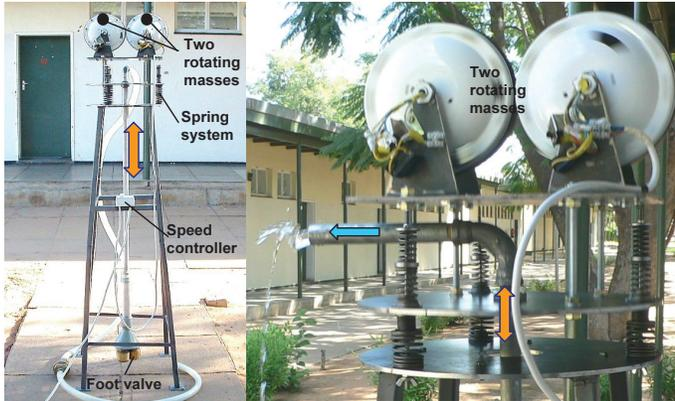
Fig. 8 illustrates the model inertial pump using the Dean Drive
