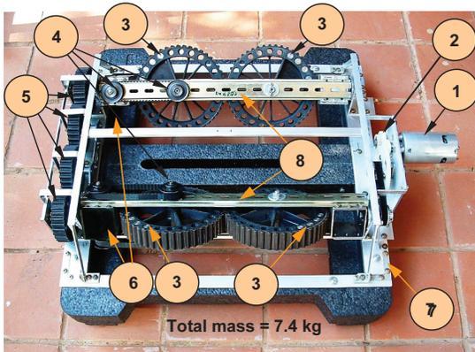
Fig. 10 shows four gyroscopic-rotors inertial drive
