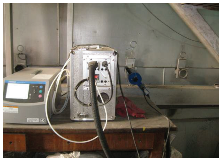
Fig.8. Horiba gas analyser location for NO x data acquisition from the end of the flame
