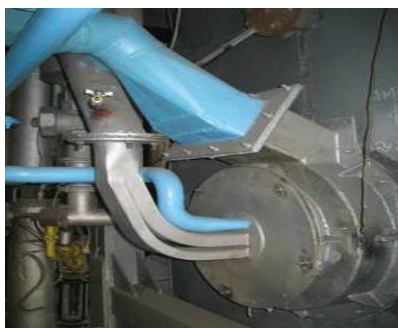
Fig.2. Staged combustion burner, functional model used in experiments
