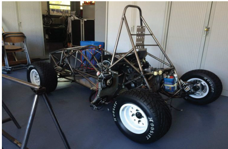
Fig.2 HFS spaceframe with suspension and engine attached
