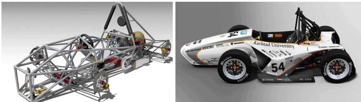
Fig.1 Formula Student Vehicle - construction and final result
