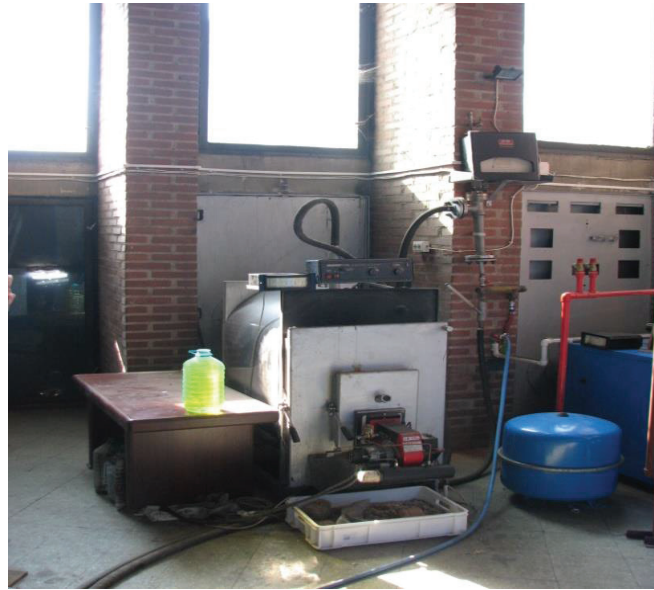
Figure 2. Experimental pilot boiler mounted to water supply system and exhaust flue
