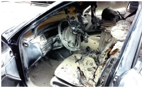
Figure. 3 Fire in a car arisen from inside the vehicle
