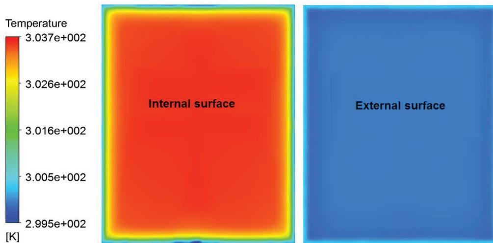
Fig. 2. Temperature fields in IGU with uncoated glasses, July 9:07 h.
