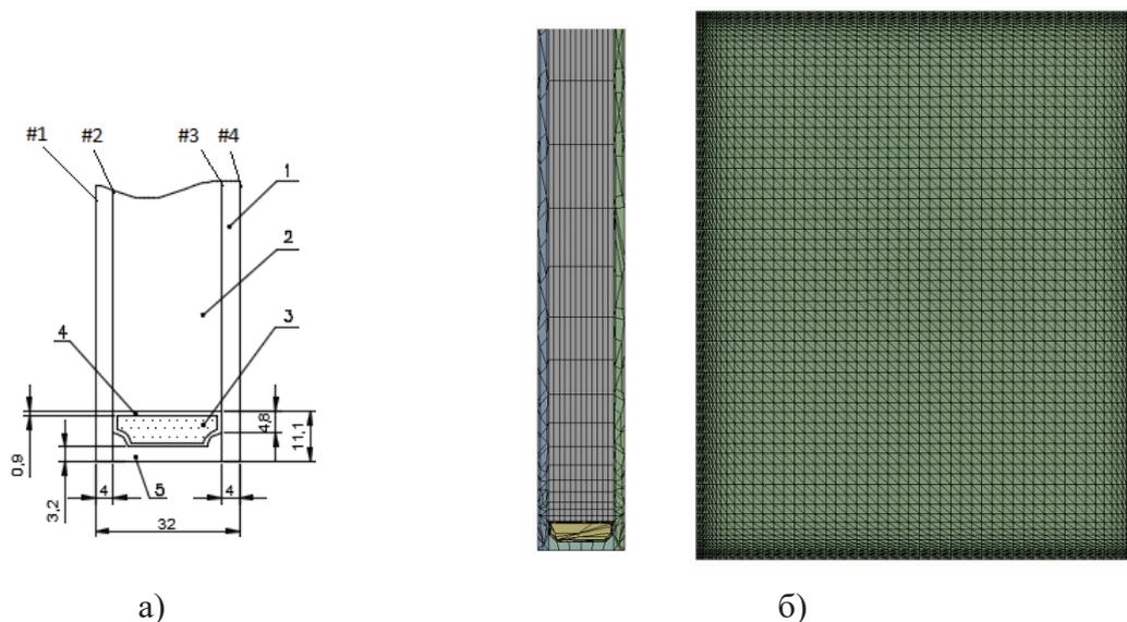
Fig.2. Double glazed insulating glass unit: a) Cross section б) Finite volumes mesh
