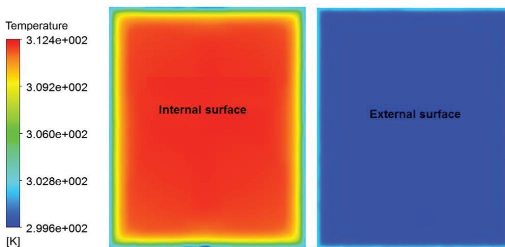
Fig. 3. Temperature fields in IGU with coating on the internal glass, July 9:07 h.
