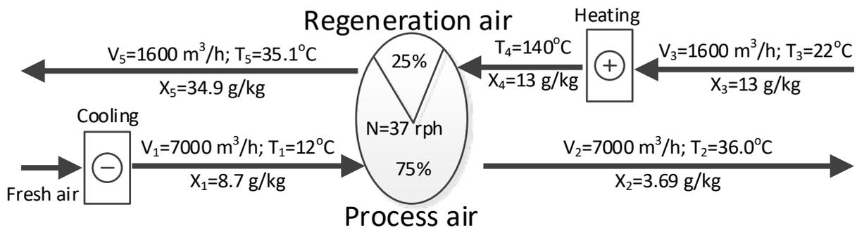
Fig. 1. Design parameters of the desiccant wheel
