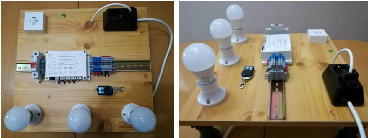
Fig. 11. Stand for remote control of lighting systems, with the use of controller "Sonoff 4Ch Pro"
