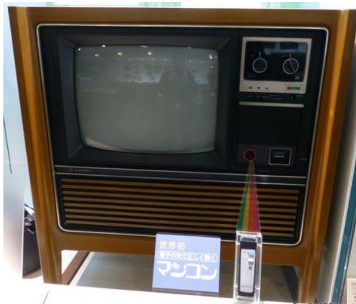
Fig. 4. Matsushita's first Colour Television with Infrared remote control National TH-6600FR
