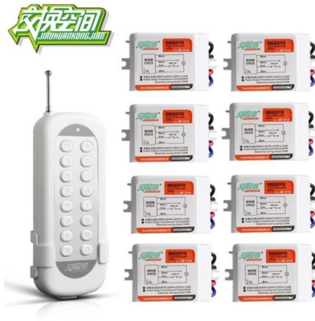
Fig. 6. Remote control of separate light sources, with separate actuators
