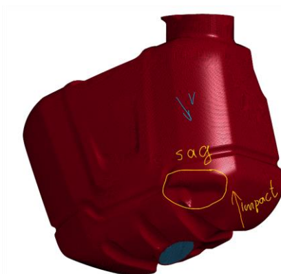
Fig. 8. A vertex impact and sagging near the vertex area.
