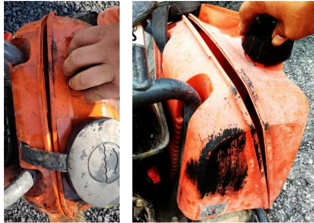
Fig. 1. Dismounting of failed tanks.
