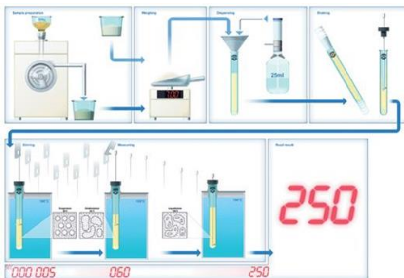
Figure 1. Scheme for measuring Falling Number (Perten, Elmer, 2020)
