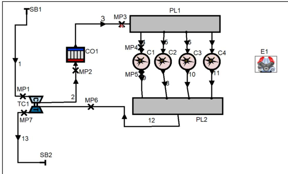
Fig. 1. Engine simulation model, developed in simulation software AVL Boost
