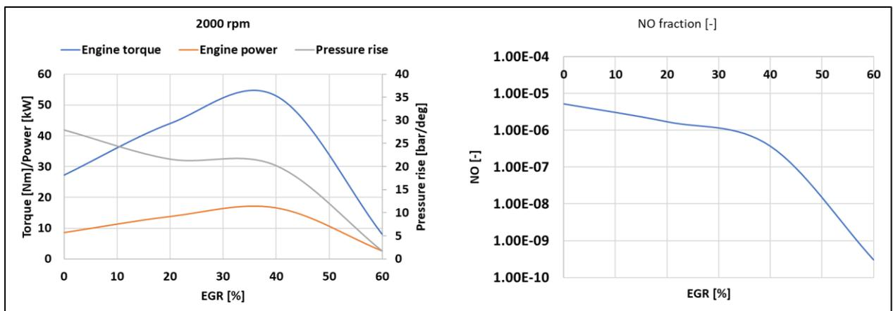
Fig. 3. Engine performance and NO fraction vs EGR rate at 2000 rpm
