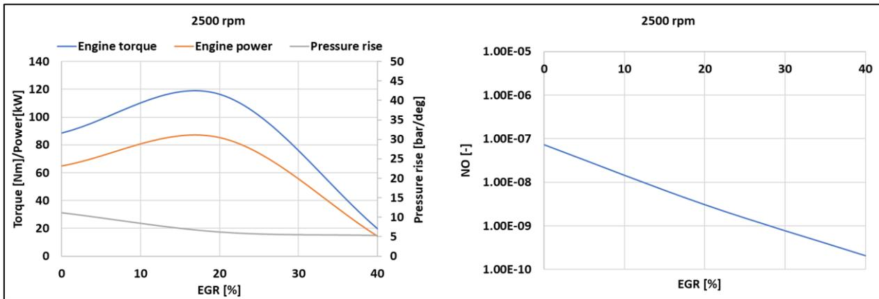
Fig. 4. Engine performance and NO fraction vs EGR rate at 2500 rpm
