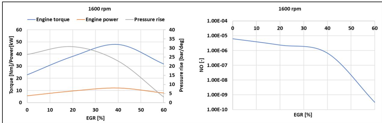
Fig. 2. Engine performance and NO fraction vs EGR rate at 1600 rpm
