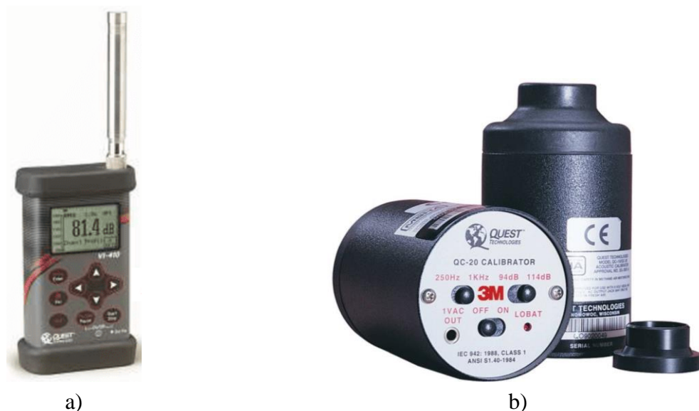
Fig.4. Measuring device VI-410 Quest Technologies a - general view; b - sound calibrator QC-10.
