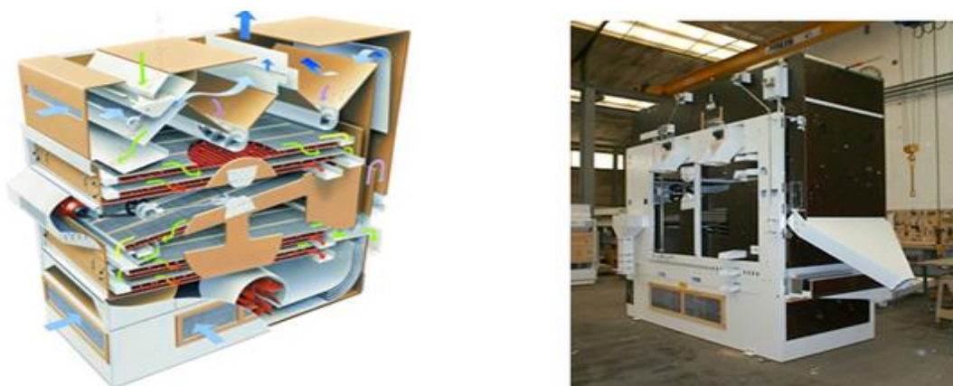
Fig. 6. Separation of different fractions of impurities
