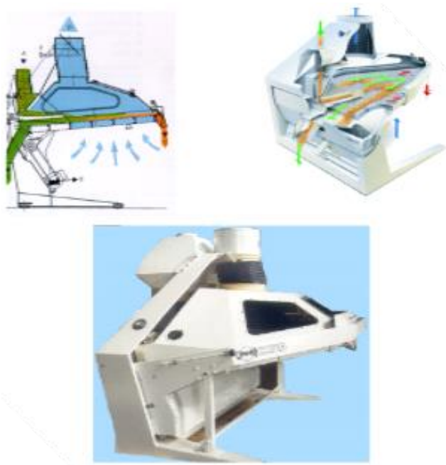
Fig. 7. Separation of stones and other inert impurities
