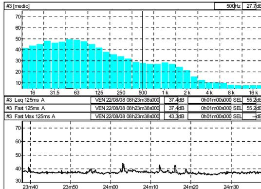
Figure 14: Electric four wheel vehicle – Background noise.
