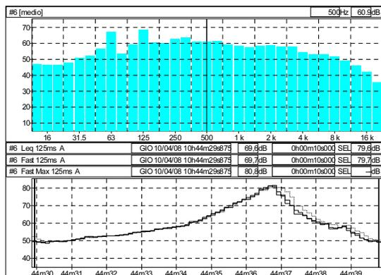
Figure 10: Traditional two wheel vehicle – Speed of 50 km/h (right side).
