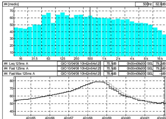
Figure 9: Traditional two wheel vehicle – Speed of 30 km/h (right side).
