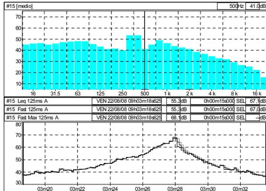
Figure 17: Electric four wheel vehicle – SEL on gradient road (right side).
