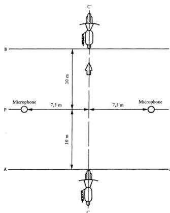
Figure 5: Test for vehicle in motion [1].
