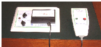
Fig. 1 Infrared Desktop Diagnostic Scanner: Meter console (left) and hand-held scanner (right). The meter console is equipped with 'sensitivity' and 'function' control knobs.
