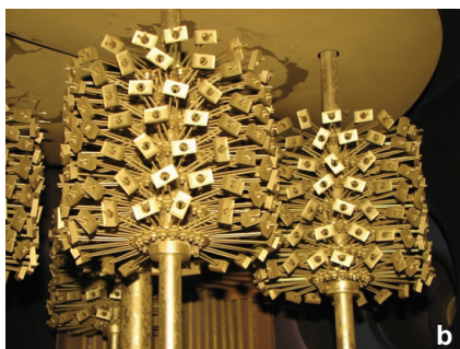
Fig. 1. Two-fold carousel movement of hard metal inserts: general look at the holder (a) and working disposition in the chamber (b).
