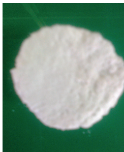
Fig. 1 – Silica xerogel prepared from sodium silicate by ambient pressure drying process
