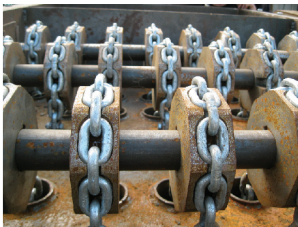
Figure 6. Ash deposits cleaning elements chain driving system
