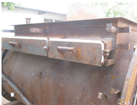
Figure 5. The position of the sliding trays for the ash deposits capturing
