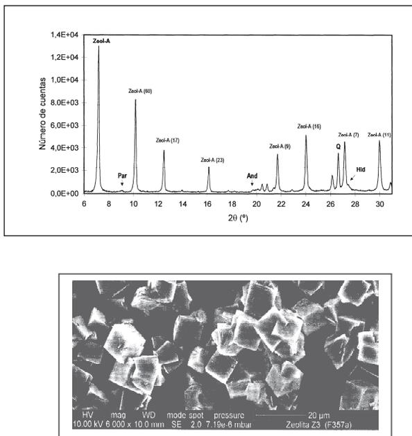
Fig. 2. XRD and SEM of zeolite NaA (composition Z<sub>3</sub>, granules)
