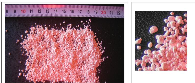
Fig. 1. Photography granules Zeolite NaA
