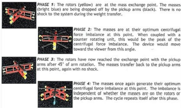
Fig. 2 shows the exchange of masses in the CIP engine
