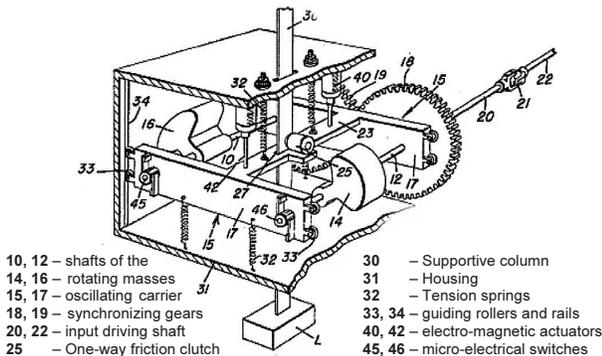
Fig. 1 displays the schematics of Dean's Drive mechanism
