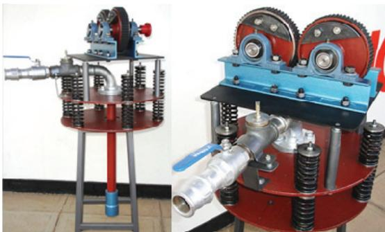
Fig. 9 displays the third prototype of inertial pump
