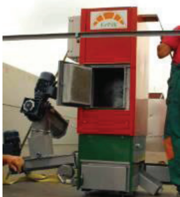
Figure 9. The 175 kW boiler
