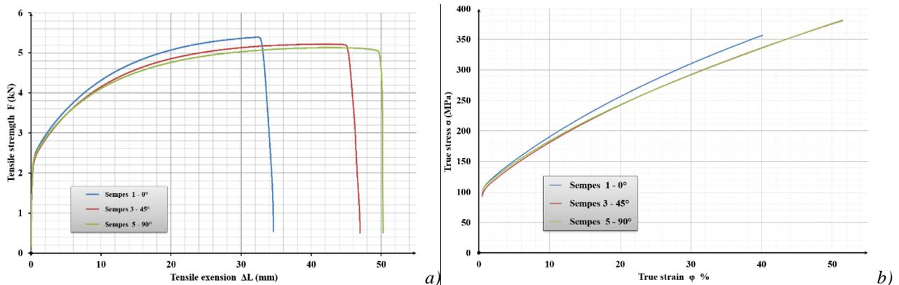
Fig. 5. Diagrams of the tested specimens of one-dimensional tensile: a) primary indicators, b) true strains and true stress
