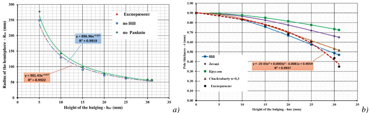
Fig. 7. Dependency of: a) radius of the hemisphere, b) the thickness at the pole in function of the height of the bulge.
