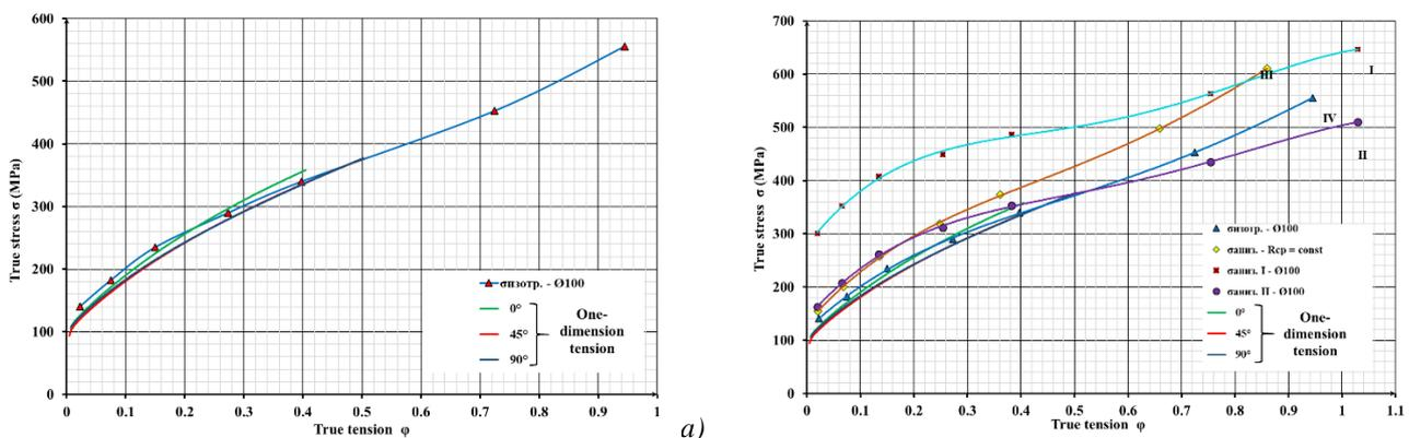
b) **Fig.8.** Curves of true tensions and true stress: a) with the premise for isotropy, b) with corrections for anisotropy.
