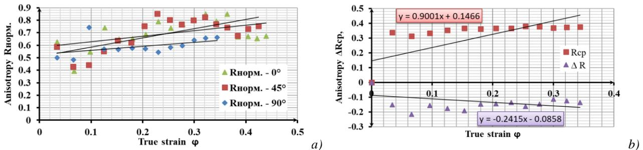
Fig. 6. Dependency of: a) normal anisotropy  $R_i$  of the degree of deformation in the three directions of testing, b) mean normal anisotropy  $R_{cp}$  and mean flat anisotropy  $\Delta\widehat{R}_{cp}$  of the degree of deformation.
