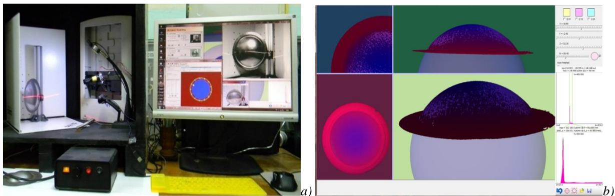
Fig. 4. System for analysis of hydraulically bulged model: a) General appearance of the 3D scanning system [19], b) Panel of the software product SA-3DSC for spherical analysis, determining the radius of the digital image and the thickness at the pole
