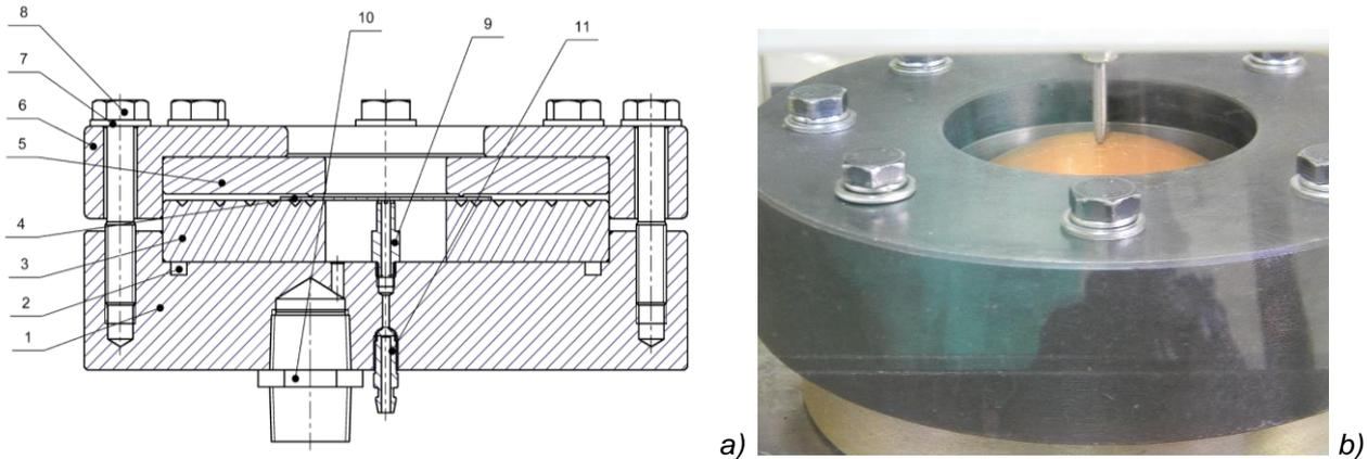
Fig. 3. Testing by hydraulic blowing of copper: a) with circular molds [19, 21, 22], b) general appearance of the hydraulic bulging
