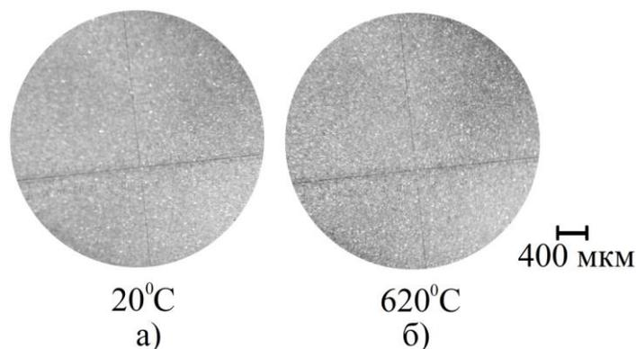
Fig. 4 Softening of the glassy bond of the experimental coating
