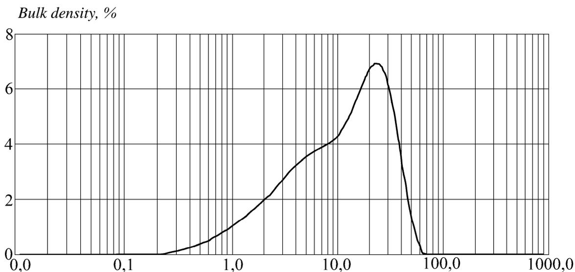
Fig. 1 Differential distribution curve of powder particles of the experimental slip
