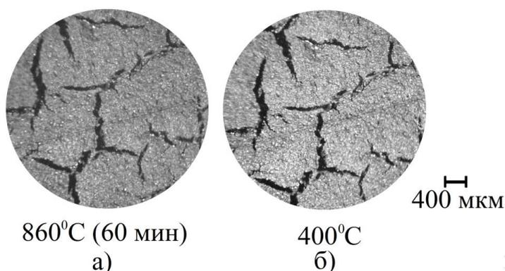
Fig. 3 Formation of the coating during isothermal exposure and subsequent cooling
