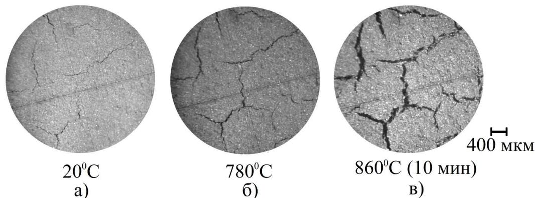
Fig. 2 Crack formation and growth of cracks in the coating
