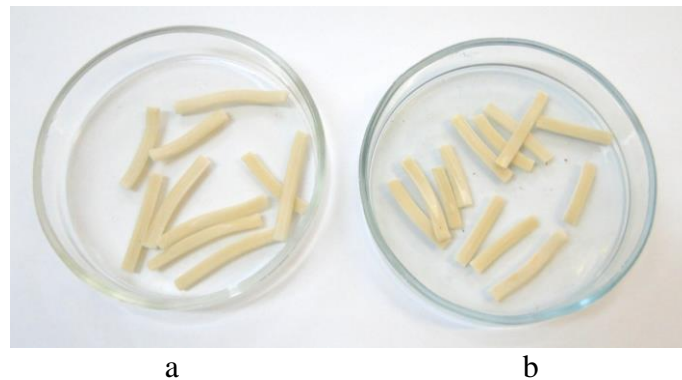
Fig. 5 Samples of obtained pasta (a – using special inserts; b – without the inserts)
