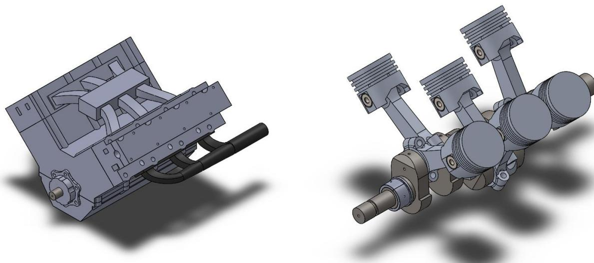
Figure 5. Isometric view of the engine taken from SolidWorks
