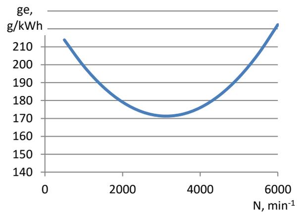
Fig. 5-4. Brake Specific fuel consumption
