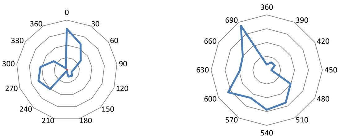
Figure 3. Polar load diagram for main bearing.
