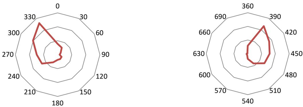
Figure 2. Polar load diagram for connecting rod big-end bearing.
