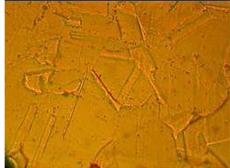
d) AISI 321, stabilized at 850°, and air-cooled, x500
