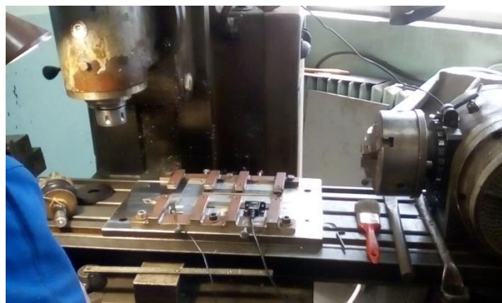
Fig. 2. “3 Axis Vernier Accelerometer” is bolted to the plate
