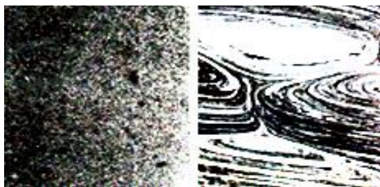
Fig. 2. Homogeneity of the material of which the PE pipes are manufactured
