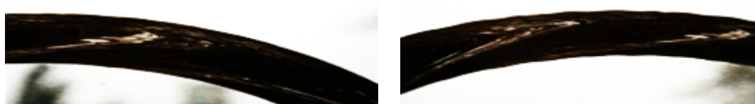
Fig. 3. Cross-section area of poor manufactured PE pipe
