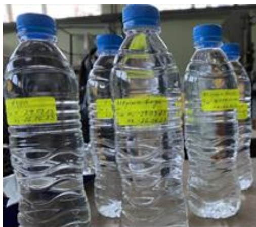
Fig. 1. Samples of PLA placed in three types of aqueous media
