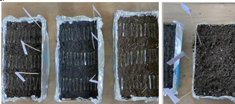
Fig. 2. Samples of PLA placed in the soil media and their covering
