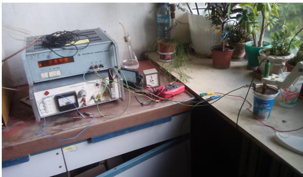
Fig. 10 Photo of the electric pretreatment of the cattle manure in Method 6
