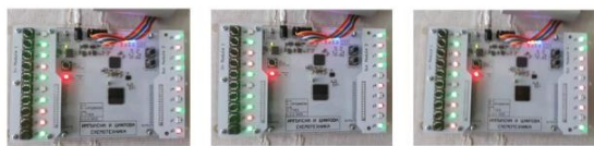
Fig. 10. Testing the magnitude comparator on the laboratory board a) 1101 > 1001 ( 13 > 9 , 1 different bit); b) 1001 < 1101 ( 9 < 13 , 1 different bit); c) 1001 < 1010 ( 9 < 10 , 2 different bits)
