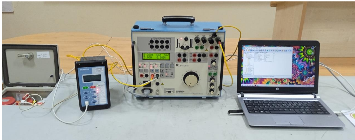
Fig. 3. Experimental setup for research and testing of the Argus 7SR10 protection relay
