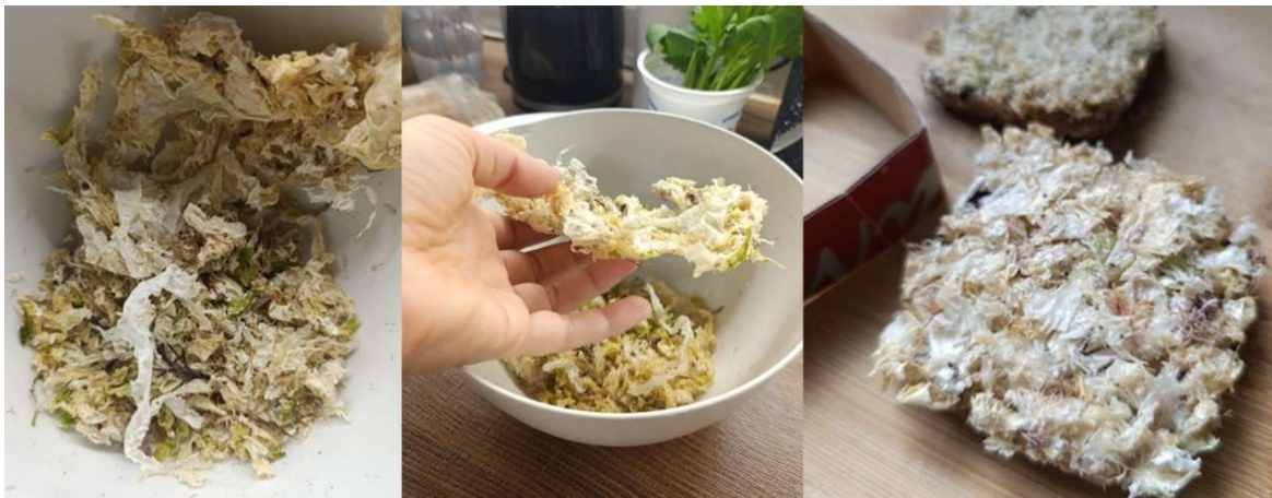
Fig. 5. Mechanically cut mixture of Black Sea algae. First attempts to obtain insulation material, sample. Photos: personal archive
