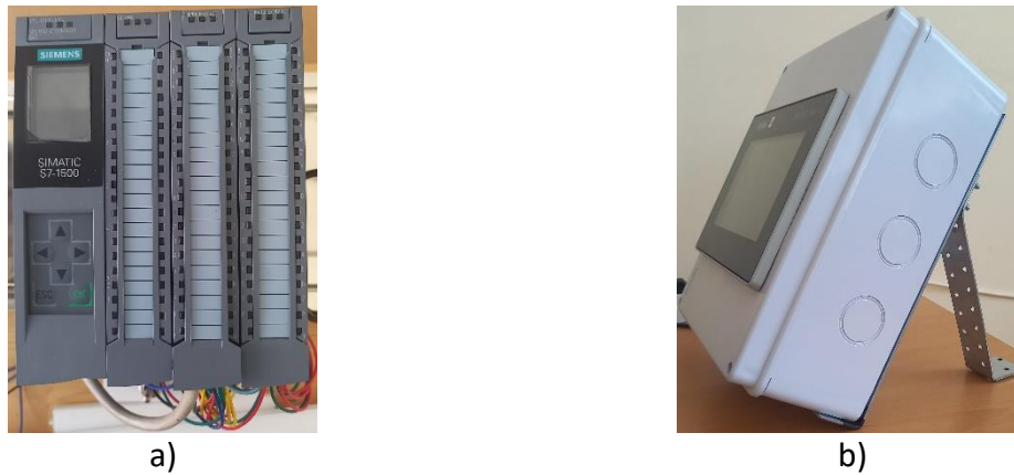
Fig. 2. New Siemens industrial equipment: a) PLC S7-1500; b) HMI
