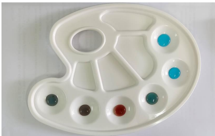
Fig. 5. Results from Benedict's test with different carbohydrates – from left to right: galactose, glucose, fructose, lactose, sucrose and starch
