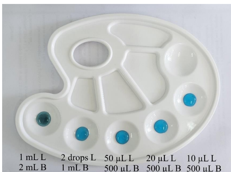
Fig. 2. Oprimization of the reagents in the Benedict test (L – lactose, B – Benedict's reagent)
