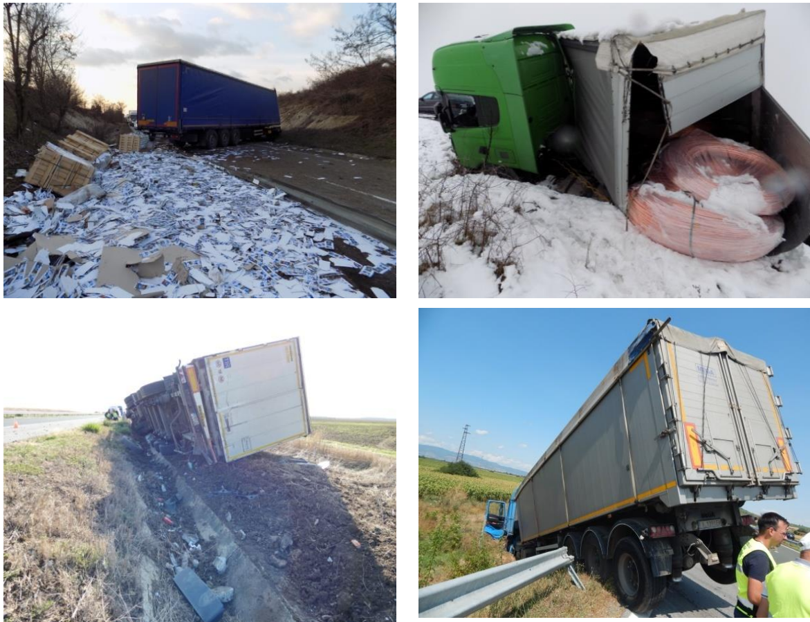
Fig. 1. Road traffic accidents caused by loss of stability
