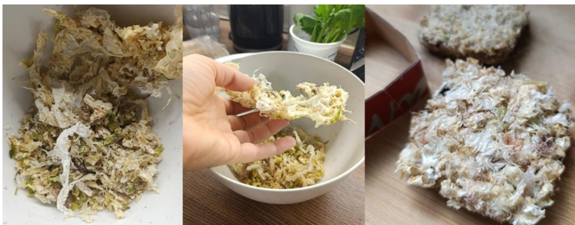
Fig. 5. Mechanically cut mixture of Black Sea algae. First attempts to obtain insulation material, sample.
