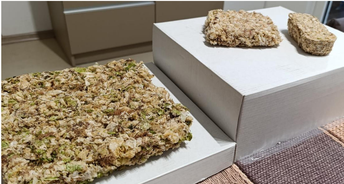
Fig. 6. Variants of insulation materials made from Black Sea algae, samples. Photos: personal archive
