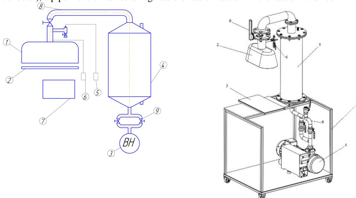
Fig. 1. Scheme of laboratory installation: 1 - vacuum chamber; 2 - vacuum chamber cover; 3 - vacuum pump; 4 - capacitor; 5 - manometer; 6 - multimeter with thermocouple; 7 - scales; 9 - pipeline.
