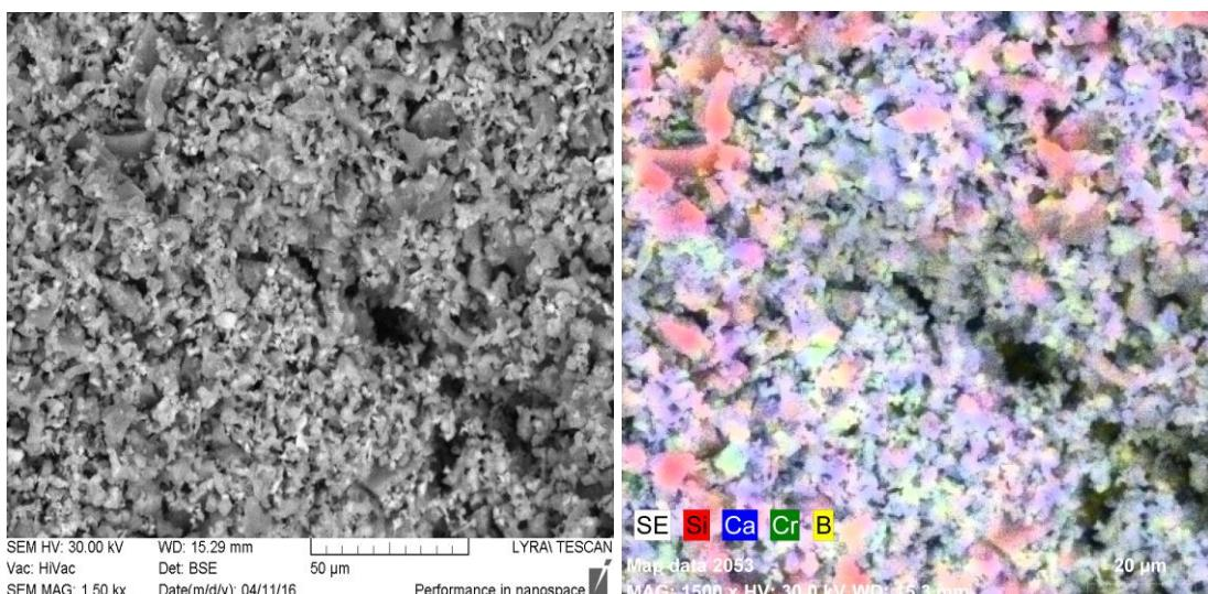
Fig. 3 Micrographs of the garnet ceramic pigments synthesized
