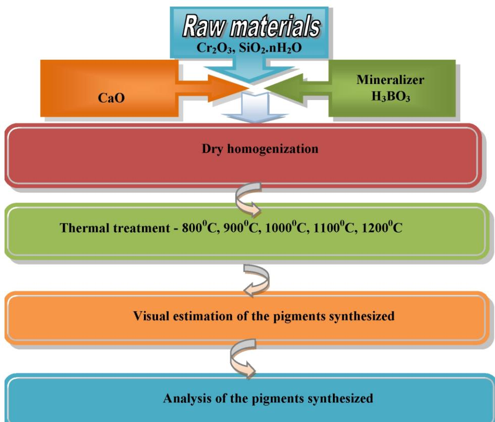
Fig.1. Technological scheme for synthesis of pigments
